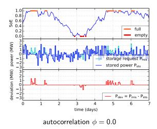
Fixed parameters: input amplitude  $\sigma_P = 1 \text{ MW}$ , capacity  $E_{rated} = 15 \text{ MWh}$
