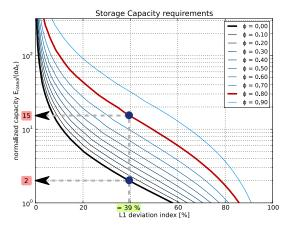
Reading as (pre-)sizing table:  $E_{rated} = f(||P_{dev}||_1, \phi)$
