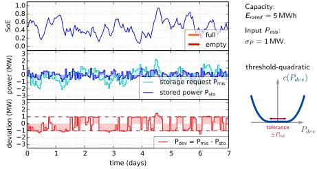
**optimal** control for a **threshold-quadratic** cost at  $\pm 1 \text{ MW}$
