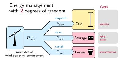
We want to **allocate** the forecast error<sup>(\*)</sup>  $P_{mis}$  between : the grid, a storage and a curtailment setpoint, at **the least cost**.
